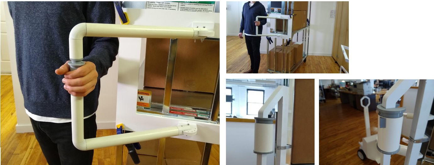
Sheath Lift UI / Spring-loaded grip falls if not lifted
